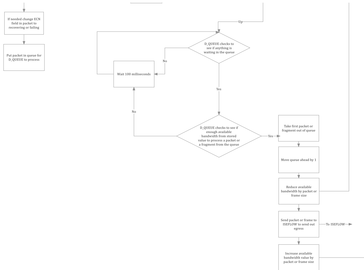
Fig. 29. Logic for processing packets in ISEFLOW with D_QUEUE, continued
