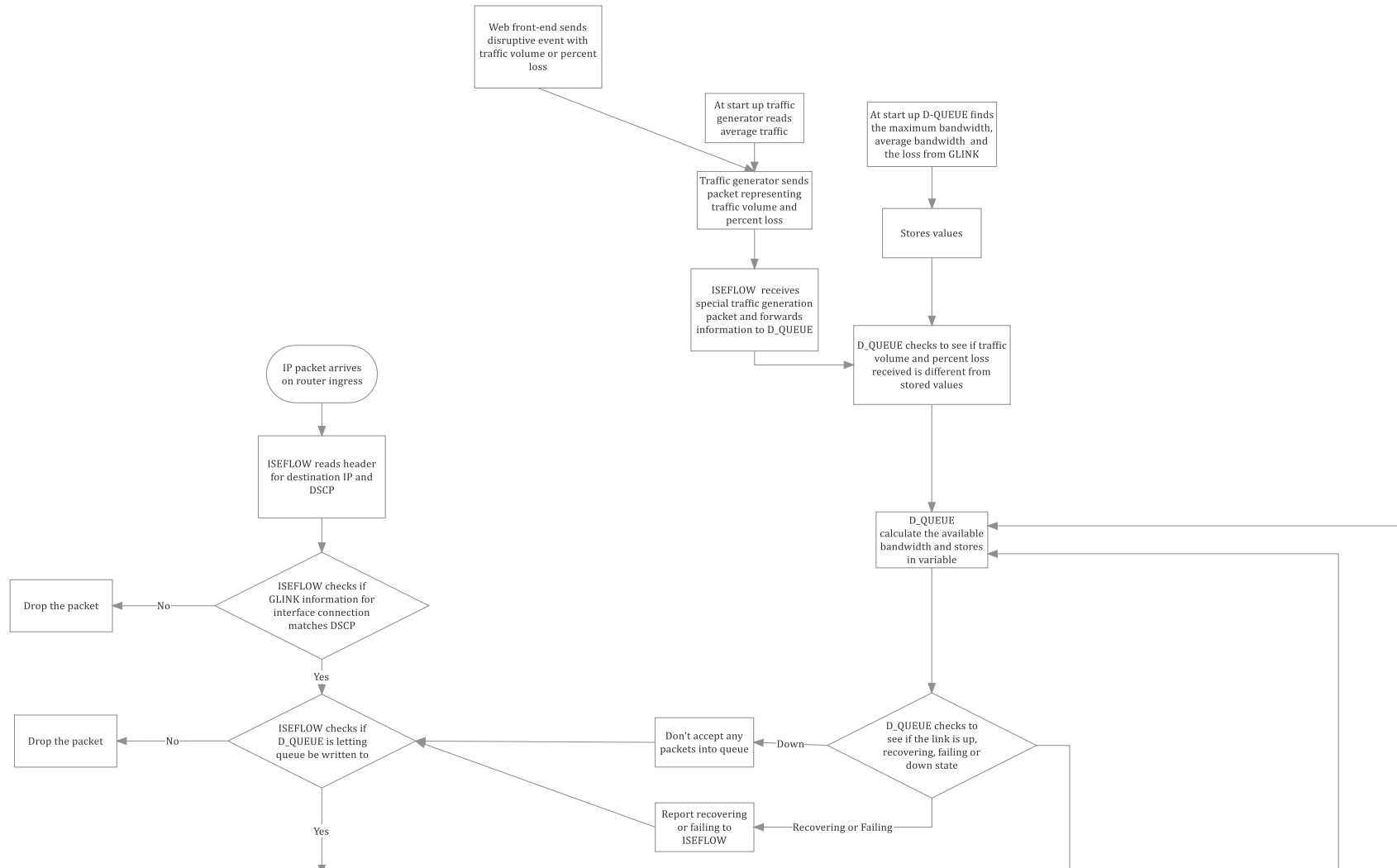
Fig. 30. Processing logic including traffic generator and disruptive event introduction
